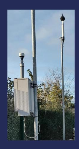
We established an environmental monitoring team for noise, air quality, dust and light pollution and enabled 37 new locations on and off Hinkley Point C site to come online to a digital monitoring system to improve noise and air quality monitoring for our Client.
